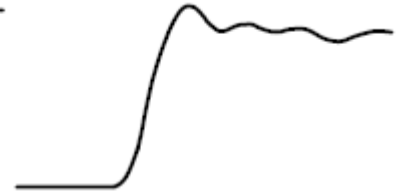
Signal with a long ground lead
