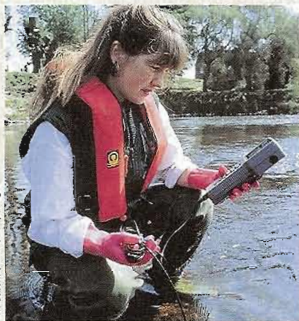
A pollution control officer measuring the oxygen content of river water.
