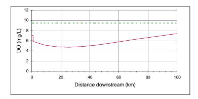
$\begin{aligned} Csat &= 9.5 \text{ mg/L} \\ k_d &= 0.23 \text{/d} \\ k_r &= 0.2 \text{/d} \\ BOD_{u,WWTP} &= 46 \text{ mg/L} \\ Q_{WWTP} &= 2 \text{ m}^3 \text{/s} \\ Q_{river} &= 10 \text{ m}^3 \text{/s} \end{aligned}$
