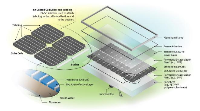
Figure 1. Diagram of the layers of a silicon solar panel (National Renewable Energy Laboratory via US EPA, 2023-b.).
