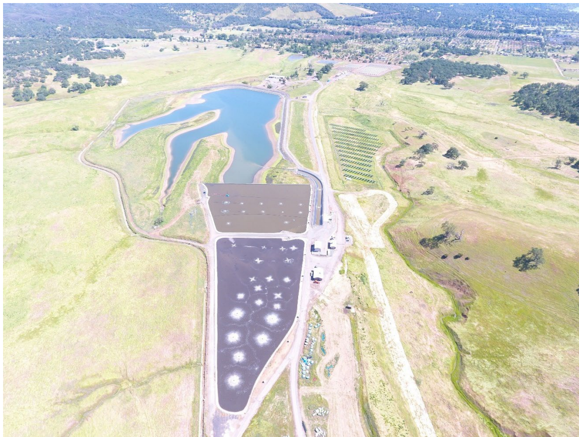
Figure 5) This is an aerial photograph looking south at the Southeast Treatment Plant. In the front is the north pond, followed by the south pond, and then discharge reservoir (Eric Luna, 2024)
