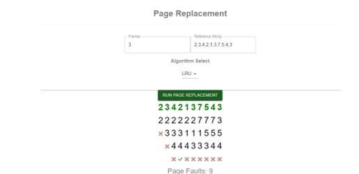
Fig. 5: A sample run of LRU replacement algorithm
