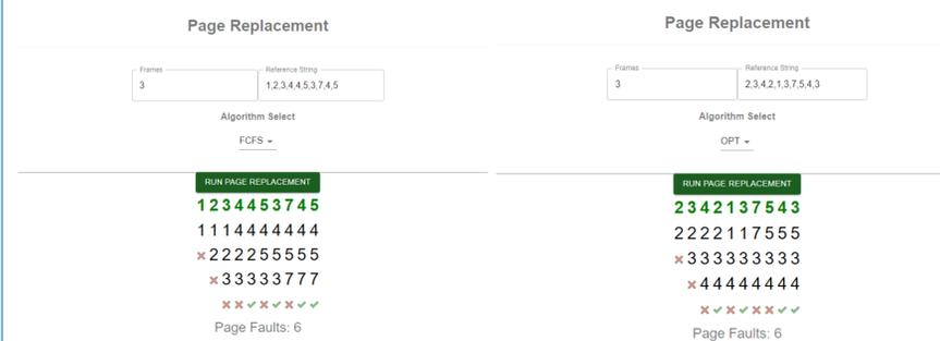
Fig. 3: A sample run of FIFO replacement algorithm
