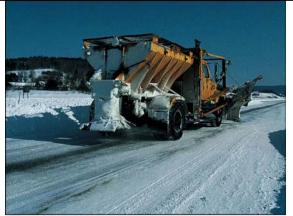
By spreading salt on the roadway, the freezing point of water is lowered, thus preventing ice formation or causing already solid ice to melt!
